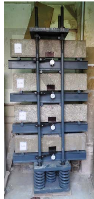
Fig. 10. Point bending creep test
