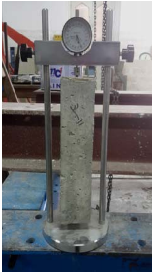
Fig 8. Free shrinkage test set-up
