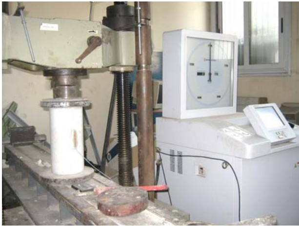
Fig. 2. Test setup of cylindrical specimens for the determination of the stress-strain relationship
