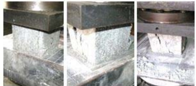
Fig. 11. Failure pattern of cube specimen (CU1)
