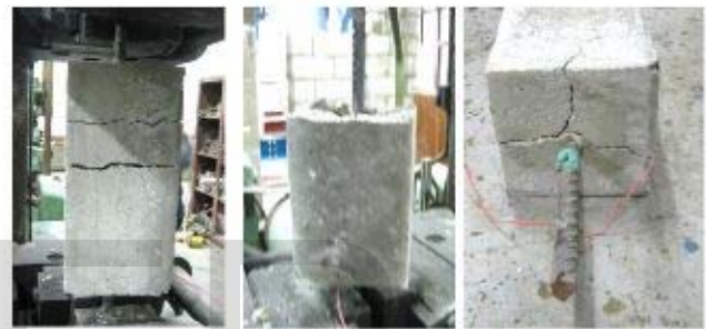
Fig. 16. Lateral cracks due to direct tension test for FBLWC
