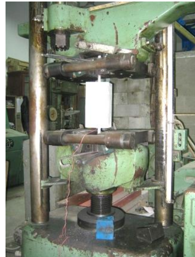
Fig. 5. Test setup for direct tension test
