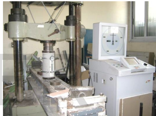
Fig. 1. Test setup for E-modulus test
