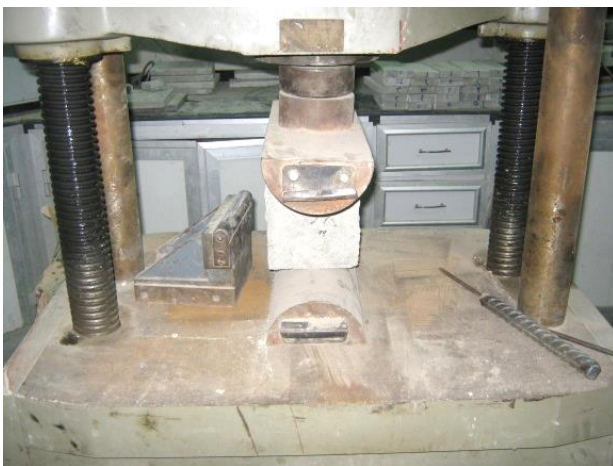
Fig. 4. Splitting tensile test on FBLWC specimens
